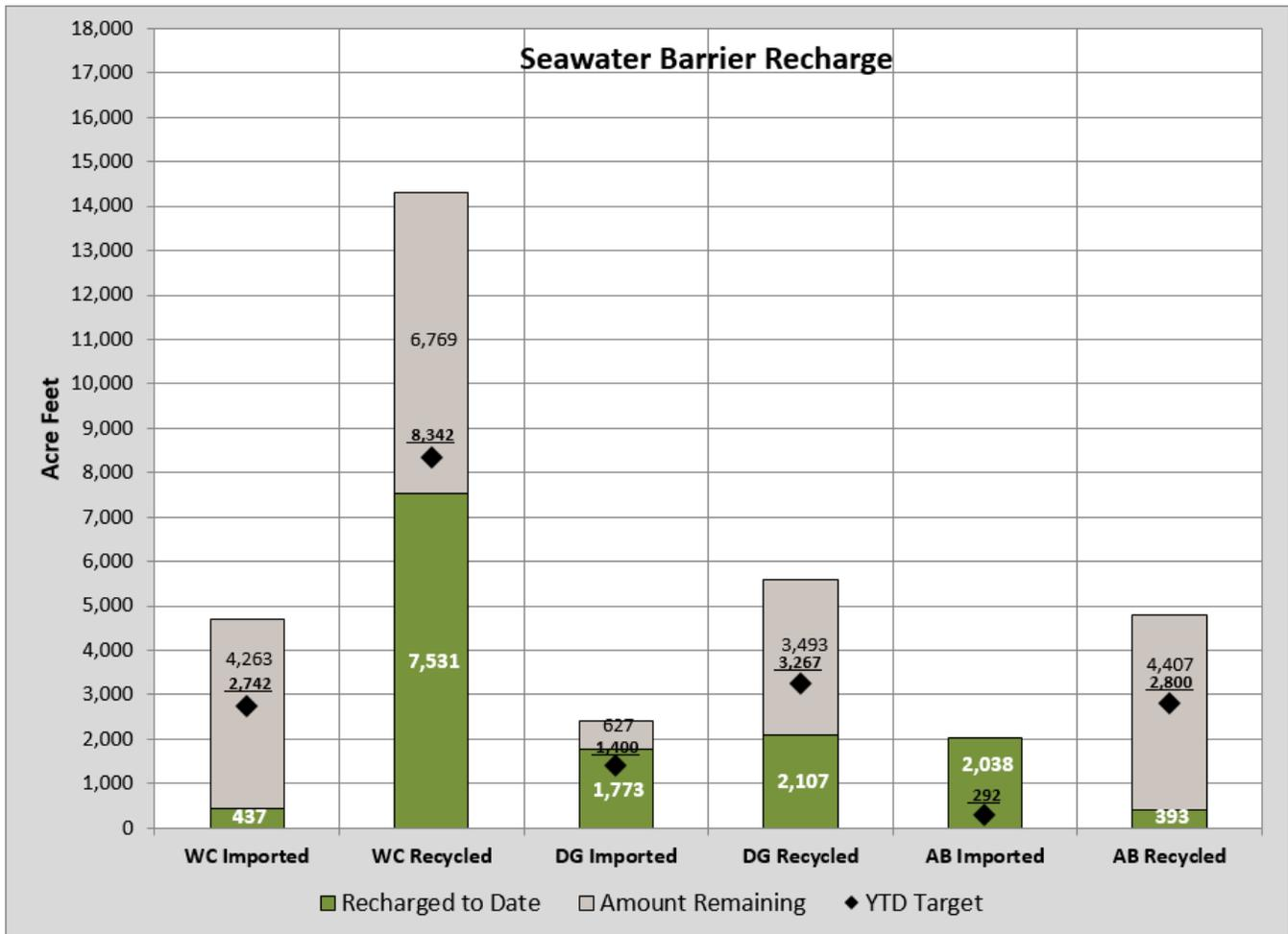
Preliminary numbers for the first seven months of the water year show that the West Coast Barrier used 437 acre-feet of imported water and 7,531 acre-feet of recycled water, or 95% recycled water. The Dominguez Gap Barrier used 1,773 acre-feet of imported water and 2,107 acre-feet of recycled water, or 54% recycled water. The Alamitos Barrier on the WRD side used an estimated 2,038 acre-feet of imported water and 393 acre-feet of recycled water, or 16% recycled water.
