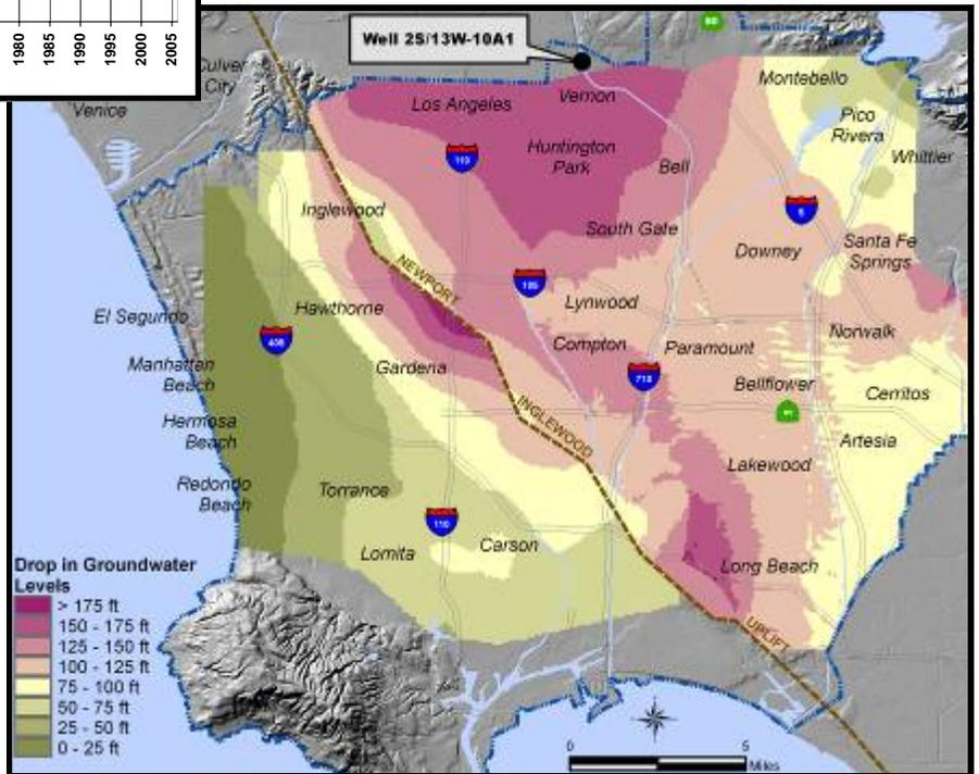
**Figure 4**—Drop in Groundwater Elevations from 1904 to 2004
