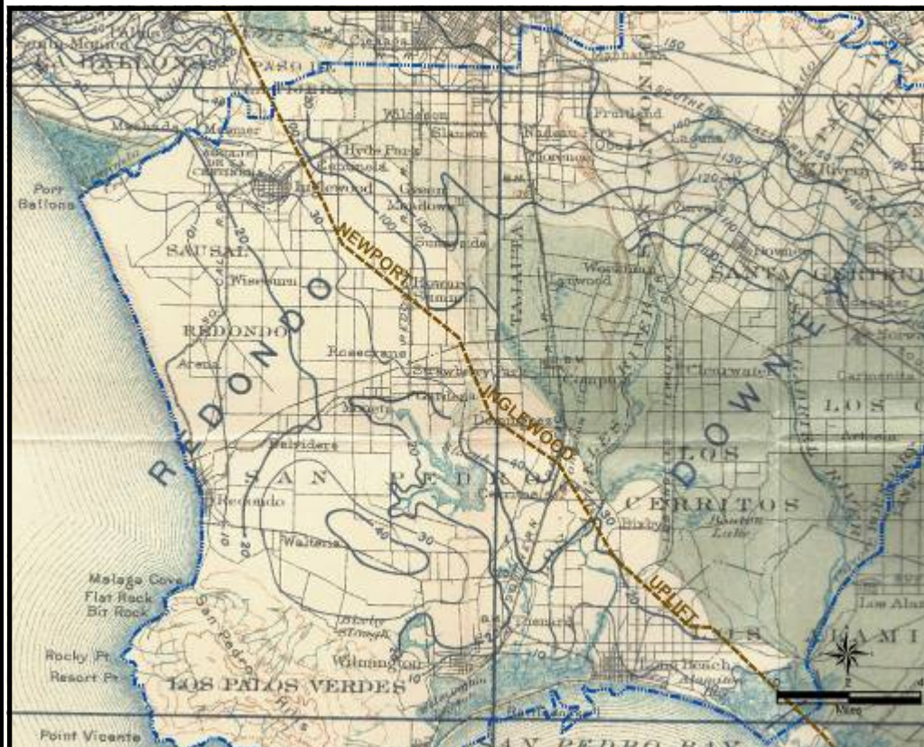
Figure 2 —Groundwater elevation contour map for 1904, modified from Mendenhall (1905). Contour values are in feet above sea level. Shaded regions in the central and eastern portions of the map are areas of flowing artesian wells. WRD boundary shown in blue for reference. Newport-Inglewood Uplift added to map for reference. Central Basin is on the east side of the uplift, and the West Coast Basin is on the west.
