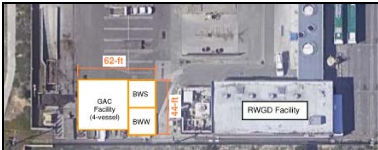
Figure 11. Site Plan for Four-vessel Granulated Activated Carbon Contactor Facility with Backwash Supply and Backwash Waste Tank and Pumping
