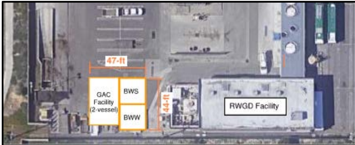
Figure 10. Site Plan for Two-vessel Granulated Activated Carbon Contactor Facility with Backwash Supply and Backwash Waste Tank and Pumping
