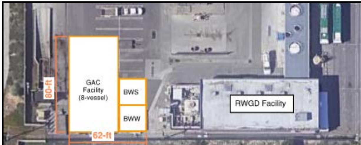
Figure 12. Site Plan for Eight-vessel Granulated Activated Carbon Contactor Facility with Backwash Supply and Backwash Waste Tank and Pumping
