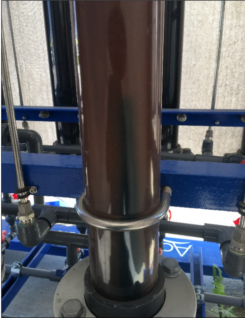
June 9, 2020, Possible algae is observed in PFA694E column. Media at MTBLW Well #7 was covered with aluminum foil
