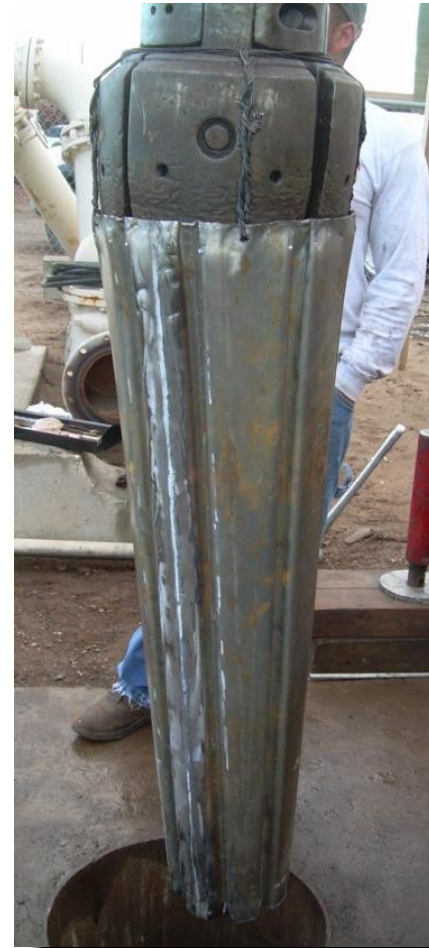
Hydraulic Swage ready to set a casing patch
