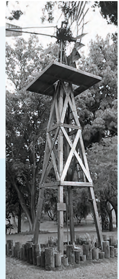
Windmill used to pump groundwater
