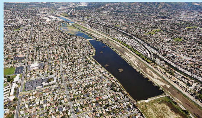
Picture of Montebello Forebay Spreading Grounds where water can filter from the surface into deep underground aquifers.
