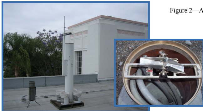
Figure 1—Automated tipping bucket precipitation station Signal Hill City Hall. Tipping mechanism shown in expanded photo at right.
