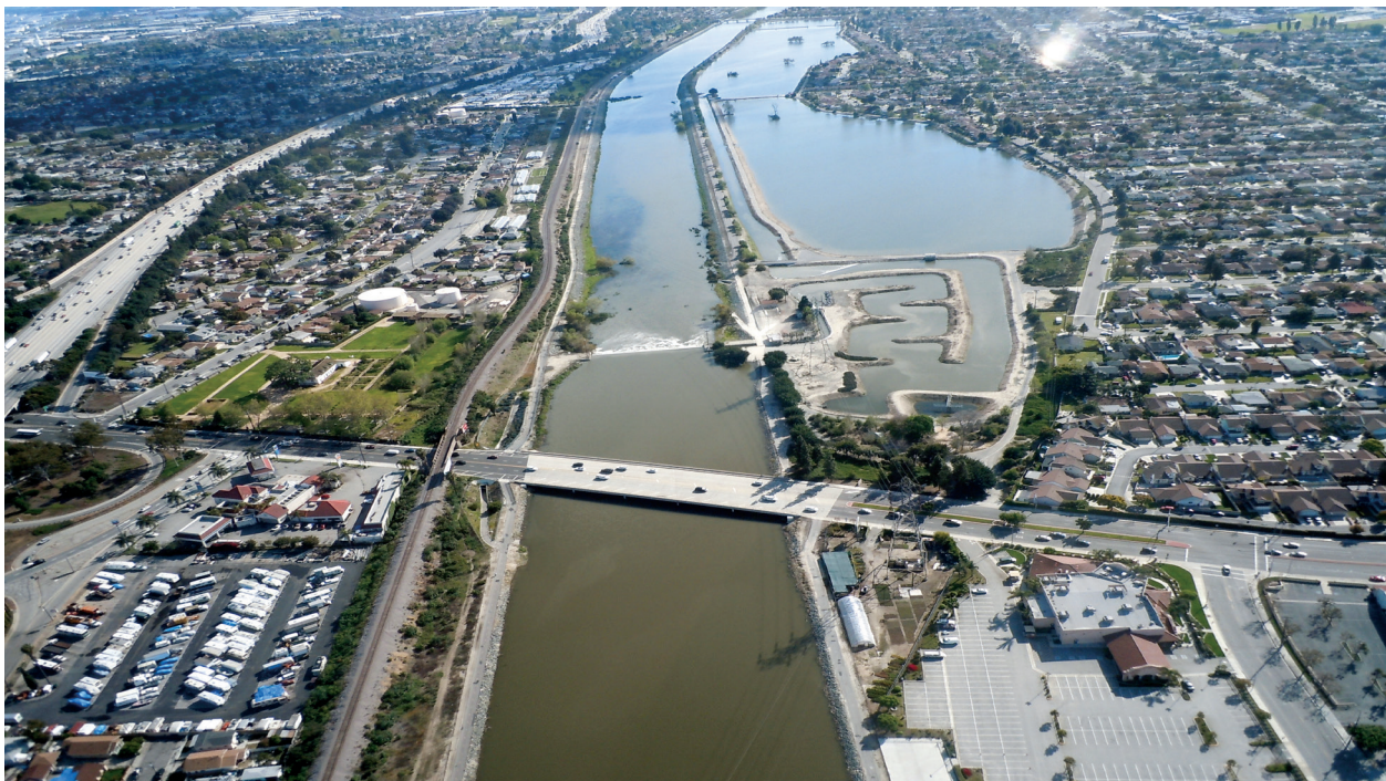
The San Gabriel River (center) and the Los Angeles County San Gabriel Coastal Spreading Grounds (right), 2011. Recycled water from the Albert Robles Center is sent through a pipeline along the San Gabriel River and is delivered to the spreading grounds for groundwater replenishment. Image from the WRD archives.
