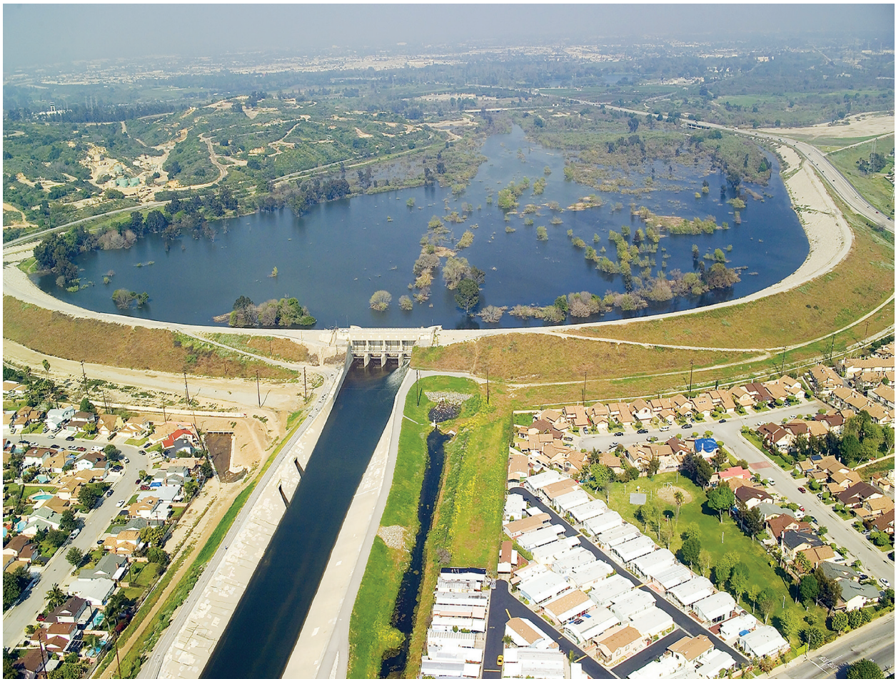
Whittier Narrows Conservation Pool, an area behind the dam that captures stormwater for groundwater replenishment, 2007. Image from the WRD archives.
