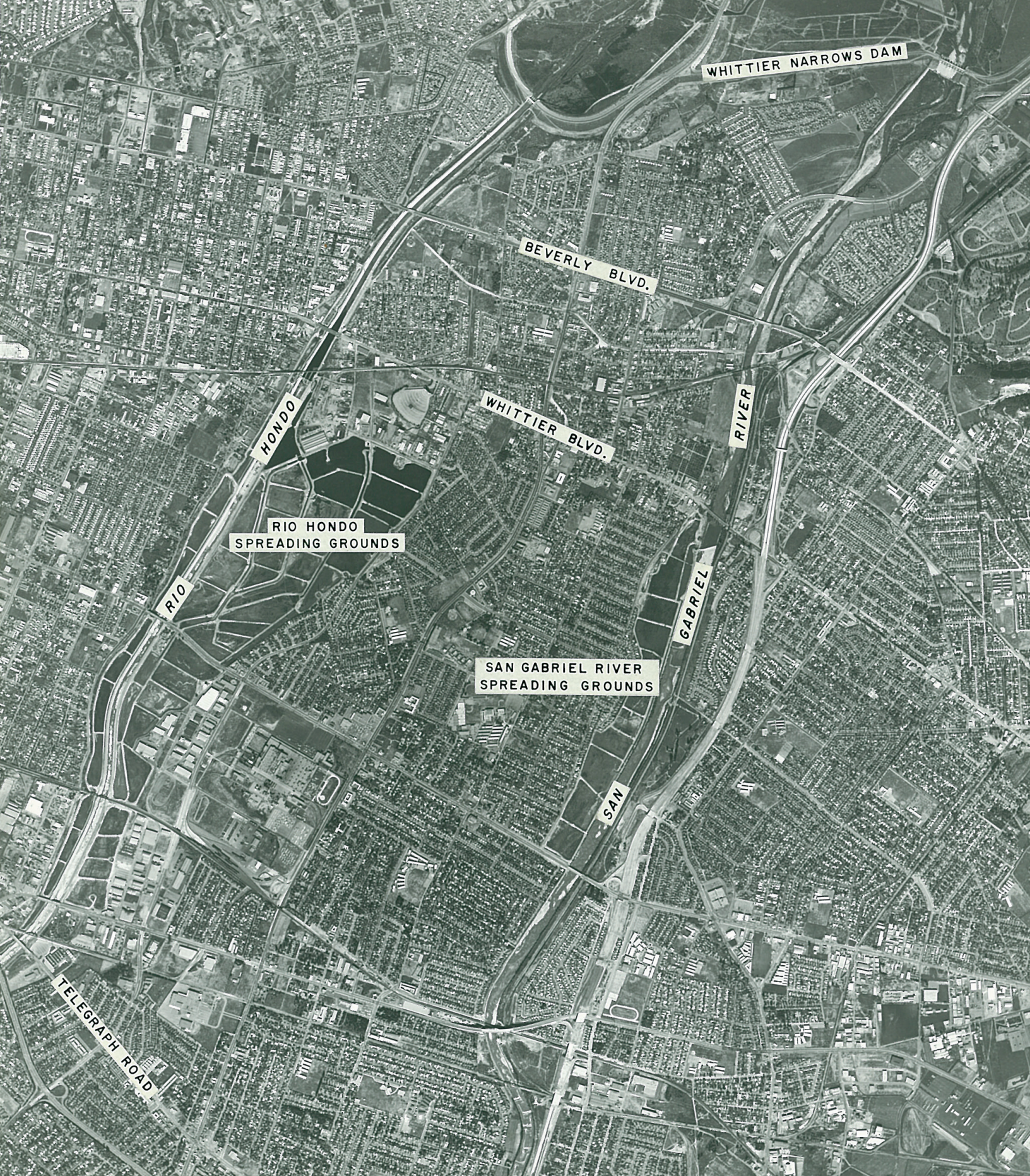
At the top of the photograph is Whittier Narrows Dam with the Rio Hondo discharging from it at left and the San Gabriel River at right. In the center of the photograph are the Rio Hondo and San Gabriel River Spreading Grounds, encompassing an area of more than 700 acres that provide the largest recharging area for groundwater in the district. Image from the WRD archives.
