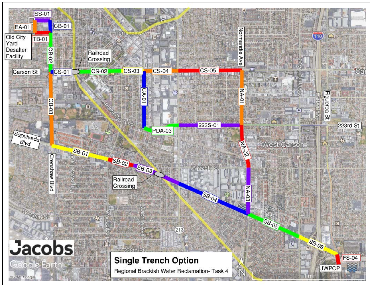
Figure 3. Single Trench Segments After Screening
